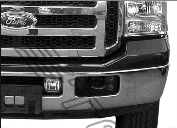
(Fig 1) Unplug wire harness behind bumper leading to fog lights if equipped
