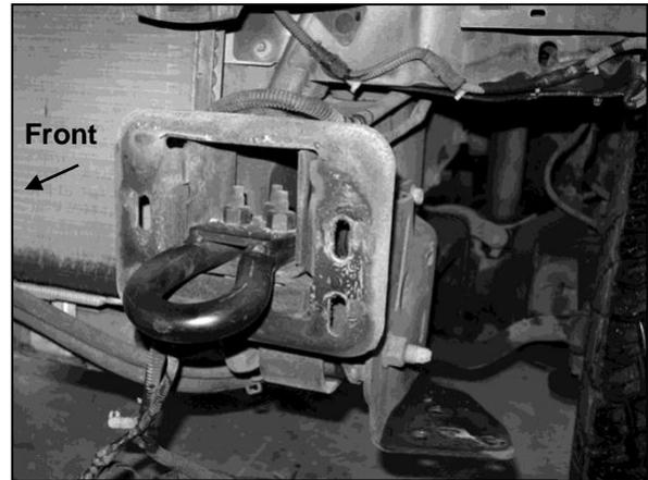
(Fig 6) Remove factory tow hook
