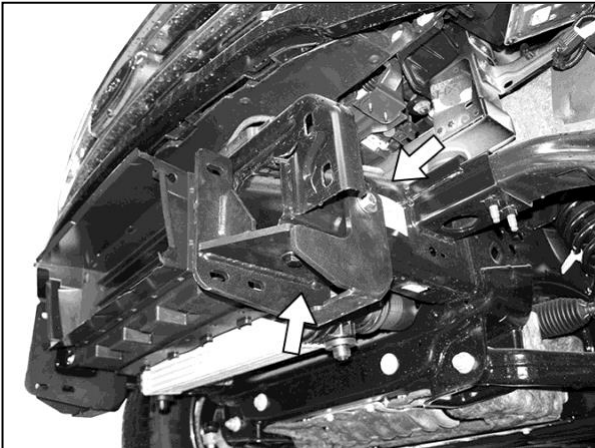
(Fig 9) Driver/left Frame Mounting Bracket attached to inner end of frame (arrows)
