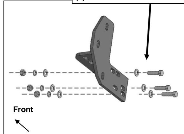
(Fig 2) Attach driver/left Frame Bracket to inside of end of frame. Line up slots in Bracket with mounting holes for factory bumper bracket
