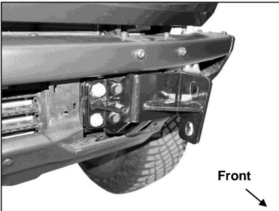
(Fig 11) Model with steel bumper, driver/left side Mounting Bracket installed
