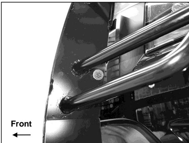
**(Fig 19) Attach driver/left Top Support Bracket to inside of Grille Guard upright**
