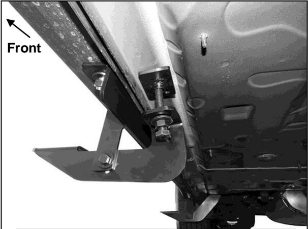
(Fig 21) Passenger/right center Mounting Bracket and Support Bracket installed
