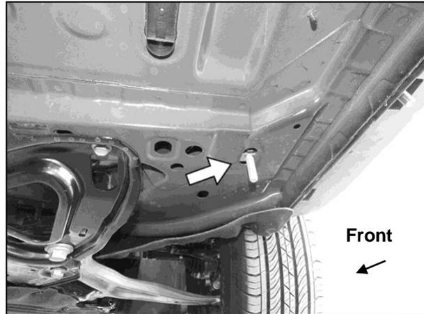
(Fig 17) Insert “Long” Bolt Plate into oval
