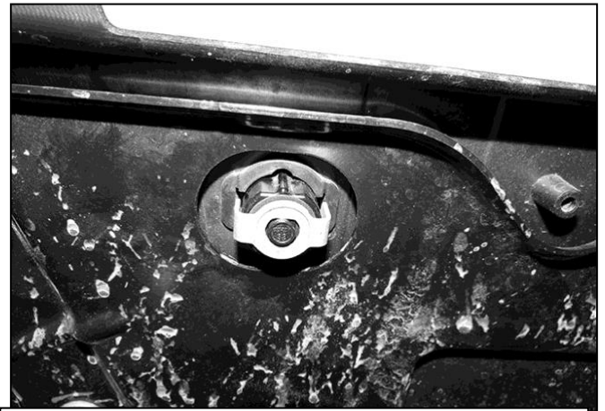
(Fig 5) Remove sensors, wire harness, trailer plug and spare tire access lock (pictured) if equipped
