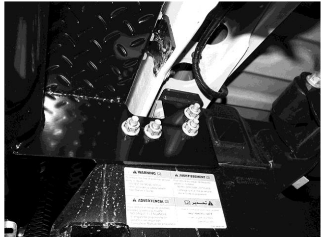
(Fig 9) Reuse factory hardware to attach passenger/right Bumper to side of frame
