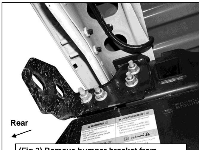
(Fig 3) Remove bumper bracket from frame. [2017-22 model year pictured]
