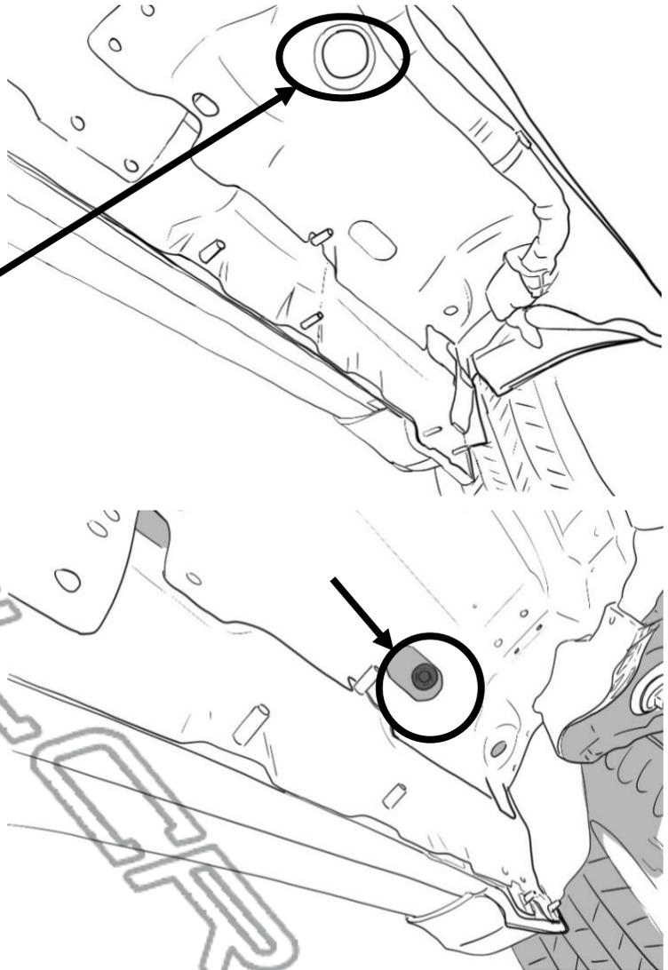
On some vehicles, the floor grommet will be a smaller rubber plug that sits inside an underside cavity. Due to the greater thickness, an incision of the plastic conduit to the appropriate branch of the power step main harness (J) may be necessary to fit through the hole.
