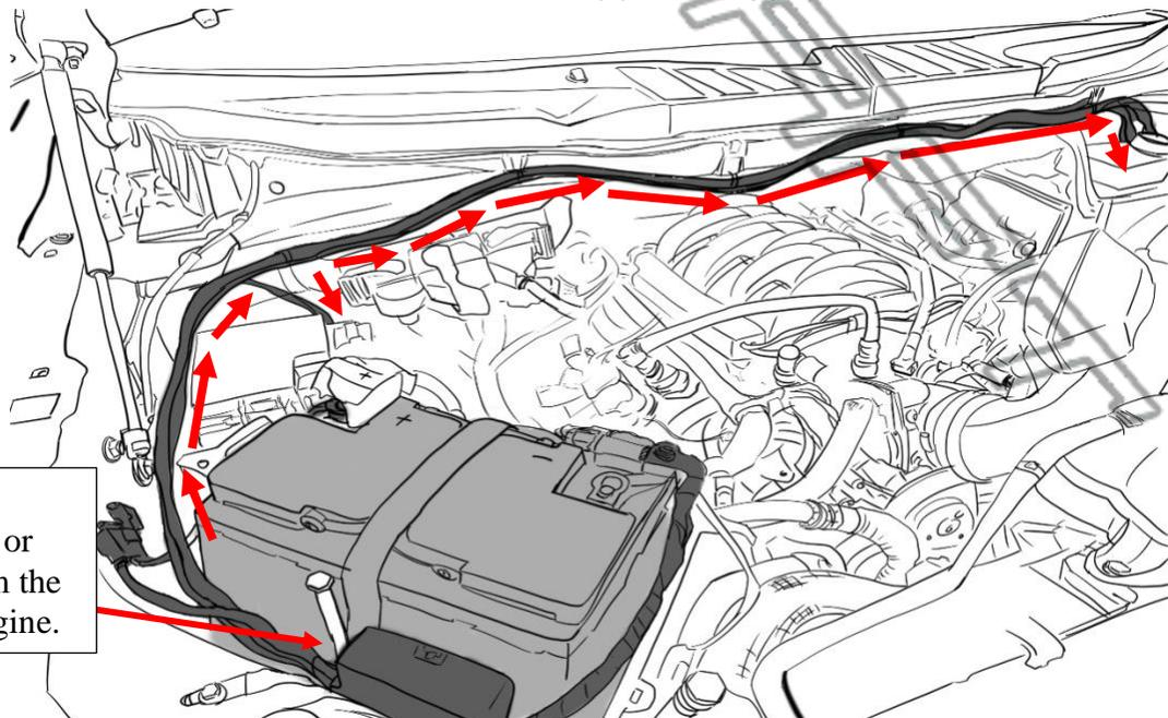
ECU (M) should be secured near battery or any space away from the direct heat of the engine.
