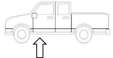
On SuperDuty vehicles, the rocker panel studs may have an OE nut already in place. Remove the nut, and then apply the plastic insulators (F) to the stud before mounting the brackets.
