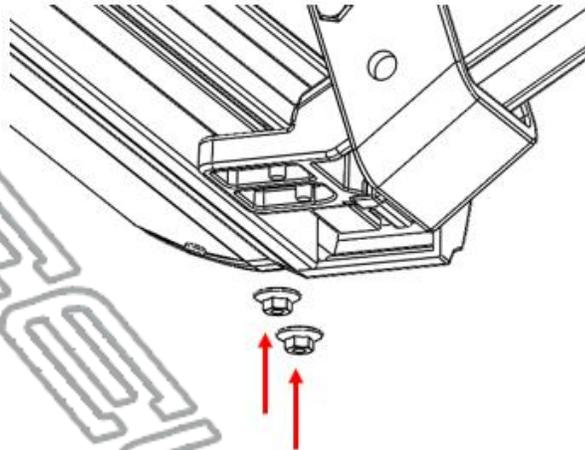
Once the board is adjusted, plug in main harness (J) connector to return power to the linkage arms. Open and close doors several times to deploy and retract the steps to settle the steps into their natural alignment. After cycling the step, tighten all hardware on the board and brackets.
