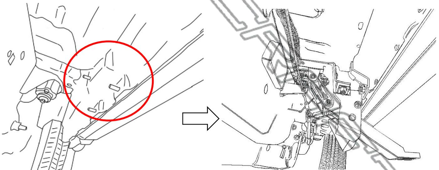
Then fasten Nylon Lock Nuts (I) and washers (H). Do not tighten all the way yet. For vehicles with e-brake cables on the Driver Side, take the rubber sleeve in the kit and slide over the brake line, near backside of the bracket assembly, to protect the line from wear. Attach sleeve to line using RTV silicone sealant.
