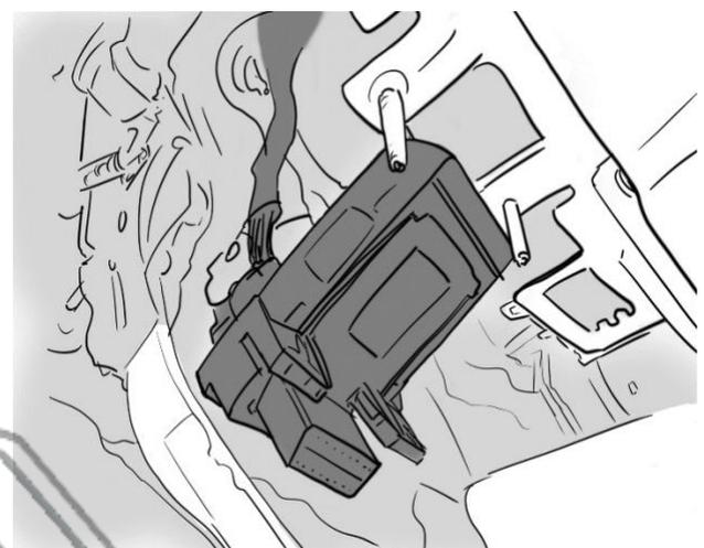
From the rear side of the connector, identify the Grey/Orange wire and Purple/Orange wire. Connect the Yellow and White wires from the Power Step Main Harness (J) using the supplied wire taps (L).
