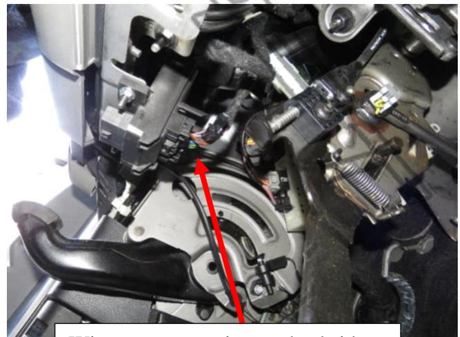
Wire taps go to wires on backside
