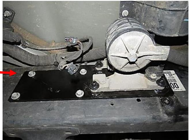
Some vehicles will have a Mass Damper instead of an ATMM. Follow the same steps and relocate the damper using the relocation brackets. Note that some vehicles will only have a mass damper on one side of the vehicle. Whenever that is the case, simply use the one appropriate relocation bracket.
