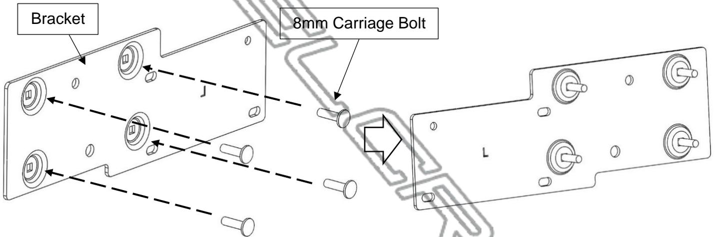
Mount the ATMM onto the relocation bracket and loosely secure into place using the provided M8 Nylon Lock Nuts (I).
