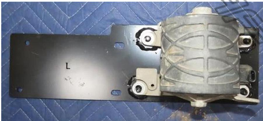
Mount the Relocation Bracket (P) onto the vehicle's Driver Side frame where the ATMM was using the OE flanged bolts. Be sure to fasten all hardware fully.
