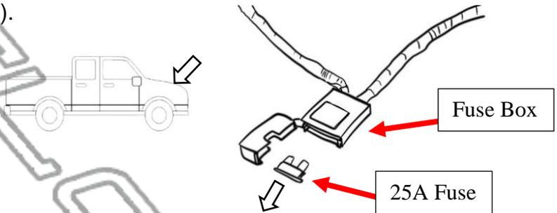
**5** Connect the positive power lead on the main harness (J) to the positive battery terminal. Connect the negative lead to the negative battery terminal.
