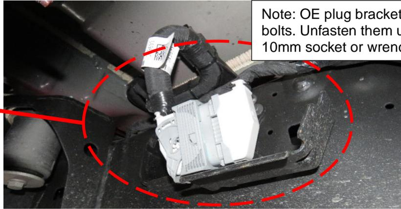
Note: OE plug bracket has 3 bolts. Unfasten them using a 10mm socket or wrench.
