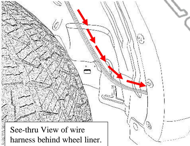
See-thru View of wire harness behind wheel liner.
