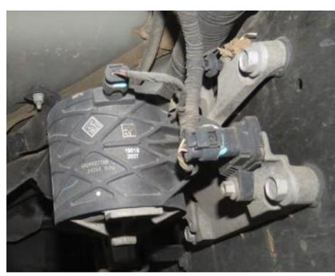
ATMM Module is meant to dampen vibrations on frame.
