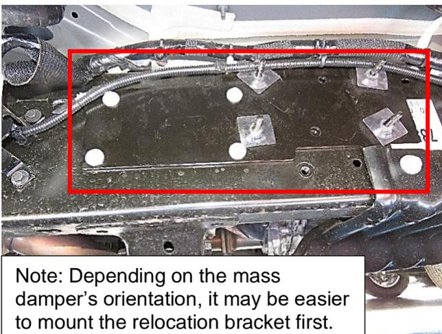
Note: Depending on the mass damper's orientation, it may be easier to mount the relocation bracket first.
