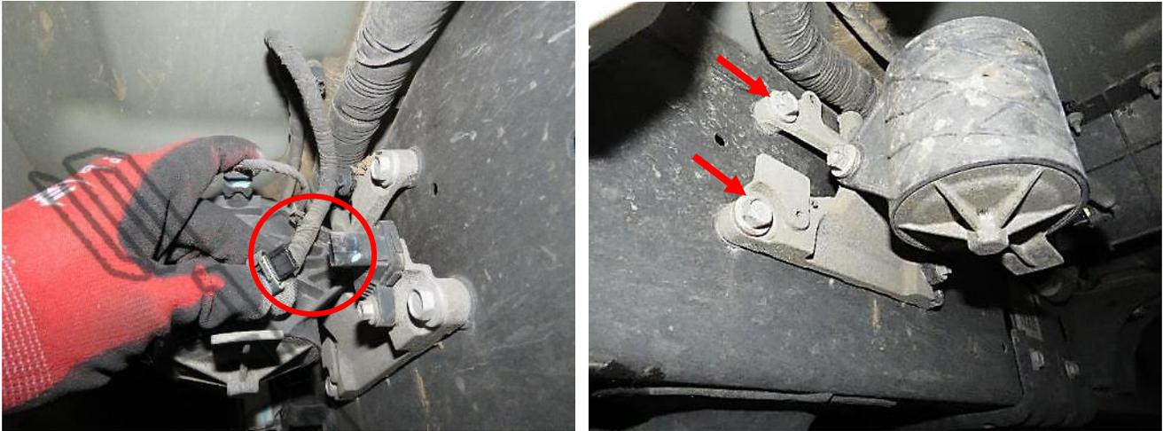
Locate Relcation Bracket (Left) (P) and M8 Carriage bolts. Insert M8 Carriage bolts (O) through the square holes on the Relcation Bracket (P) and secure using Plastic Insulators (F). This will keep the carriage bolts from falling out of the holes on the bracket.
