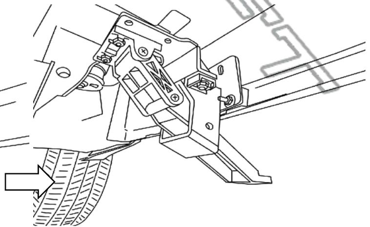
For Quad cab models, the extended rear bracket assembly (B) will shift the linkage arm position in front of the interfering vehicle frame and body mounts.
