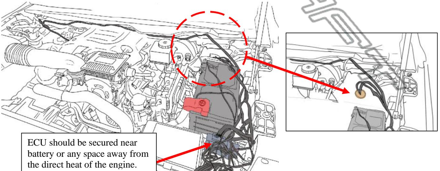
ECU should be secured near battery or any space away from the direct heat of the engine.
