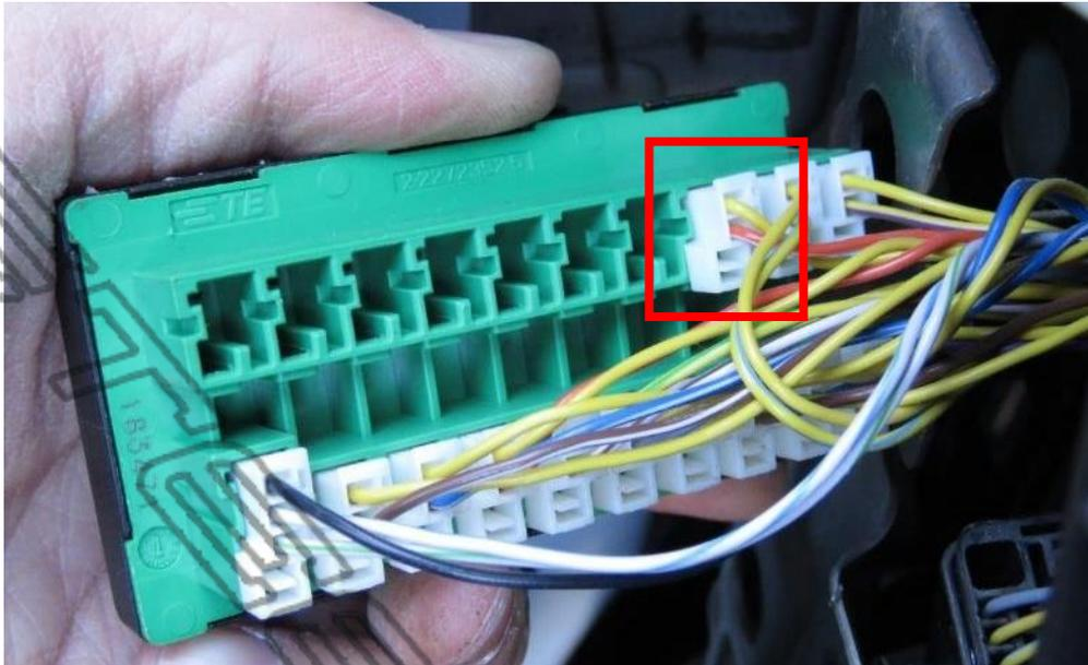
Confirm that the truck is powered off. Connect the High and Low wires from the main harness (J) using the supplied wire taps (L). After successfully connecting the wires, return the module back into its place and check that it is secure on the bracket.
