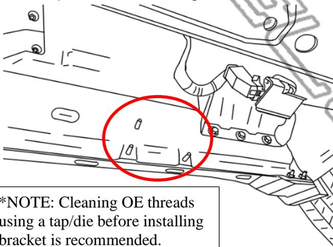
\*NOTE: Cleaning OE threads using a tap/die before installing bracket is recommended.
