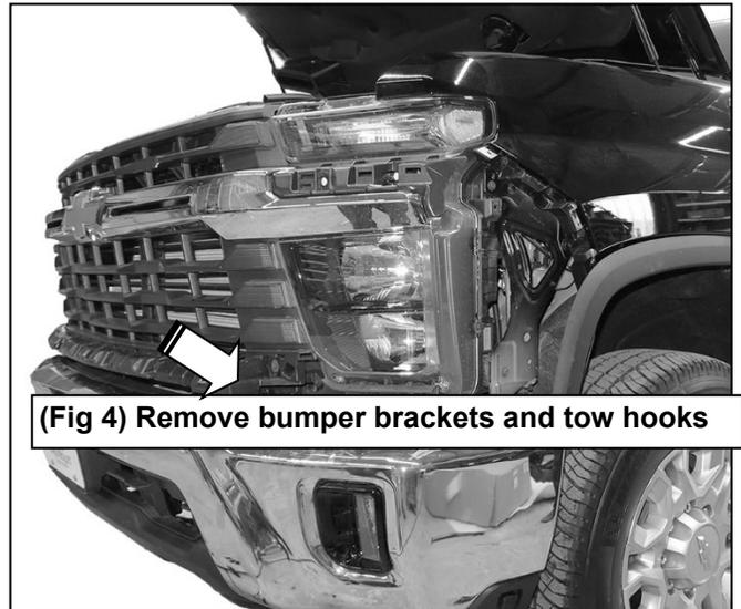
(Fig 4) Remove bumper brackets and tow hooks
