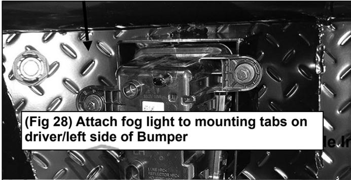
**(Fig 28) Attach fog light to mounting tabs on driver/left side of Bumper**
