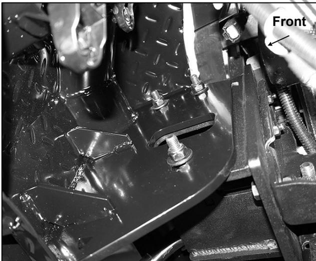
(Fig 26) Driver/left side of Bumper installed
