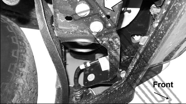
(Fig 9) Remove driver/left and passenger/right outer bumper supports attach to bottom of frame
