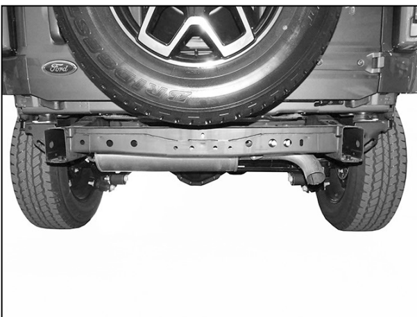
( Fig 3 ) Remove bumper assembly
