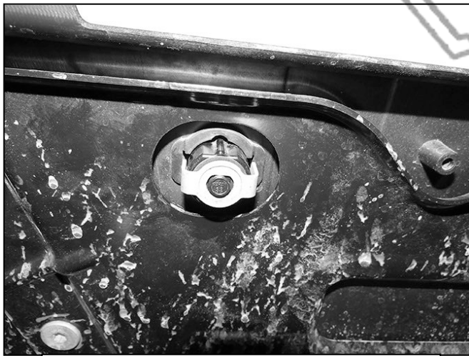
(Fig 5) Remove sensors, wire harness, license plate lights, trailer plug and spare tire access lock (pictured) if equipped
