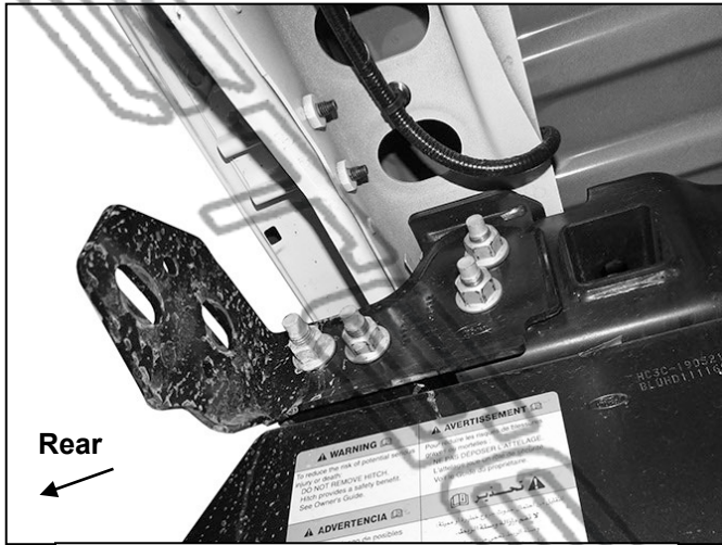
(Fig 3) Remove bumper bracket from frame. [2023-on model year pictured]
