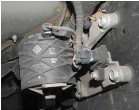
ATMM Module is meant to dampen vibrations on frame.
