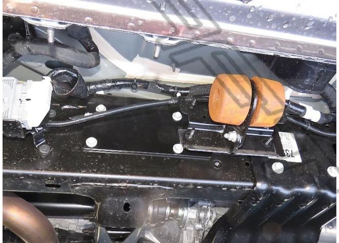
On some vehicles like the TRX, an OE module plug may be in the way. If so, unbolt the plug's bracket from the frame. Then remove the plug from the bracket. Plug may be located at the front or rear.
