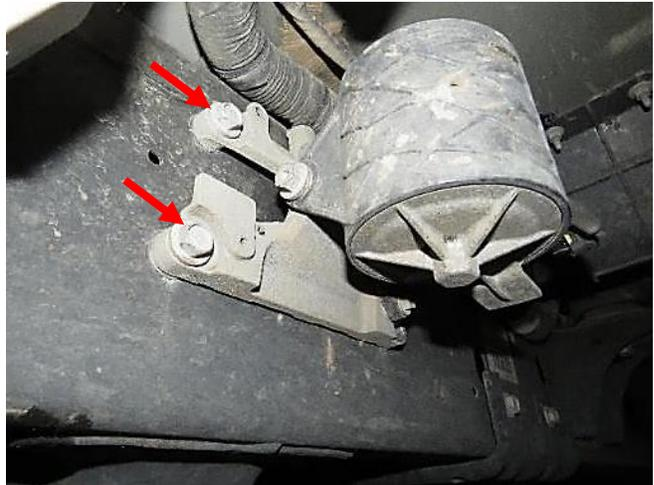
Locate Relcation Bracket (Left) (P) and M8 Carriage bolts. Insert M8 Carriage bolts (O) through the square holes on the Relcation Bracket (P) and secure using Plastic Insulators (F). This will keep the carriage bolts from falling out of the holes on the bracket.
