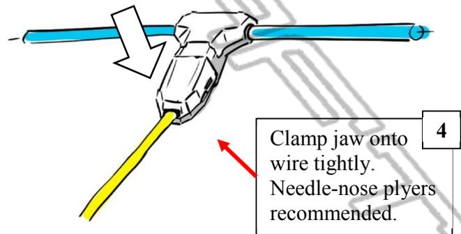
NOTE: Make sure wire is seated properly in the jaws before clamping. The wire being tapped must be centered on the “teeth” to make a proper tap.
