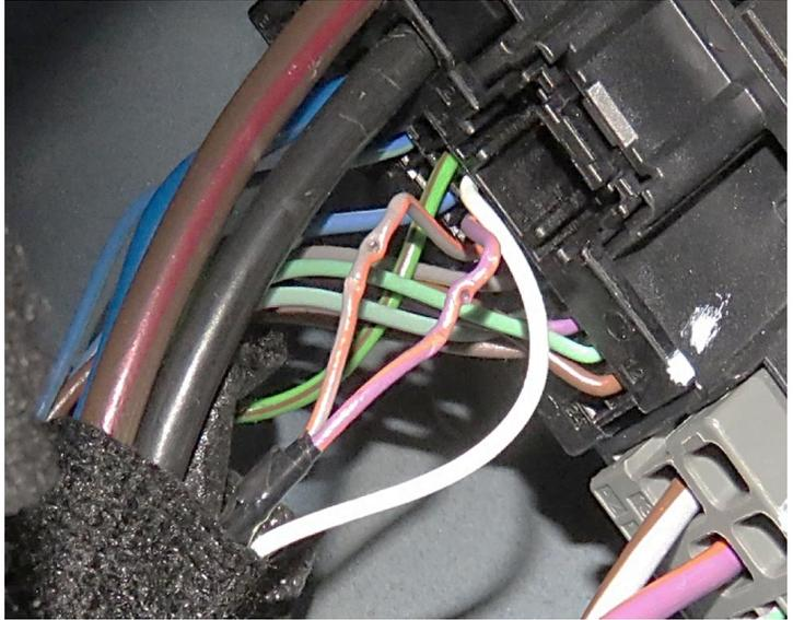
\*NOTE: If board does not move during troubleshooting, check to see if the taps tapped the wires correctly.
