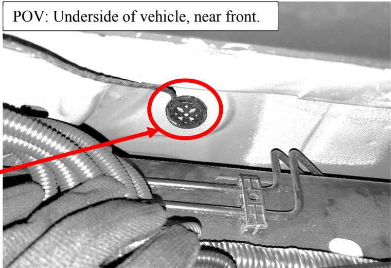
On some vehicles, it may be necessary to route through the engine bay firewall instead. In these cases, locate an oval grommet on the Driver Side of the firewall, and route through the grommet.
