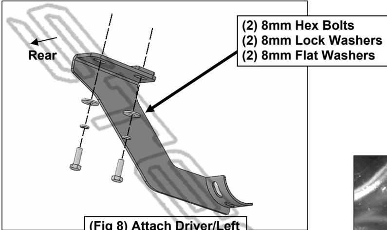
(Fig 8) Attach Driver/Left Rear Mounting Bracket
