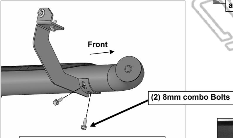
(Fig 10) Attach the Driver/Left Sidebar to the (3) Mounting Brackets
