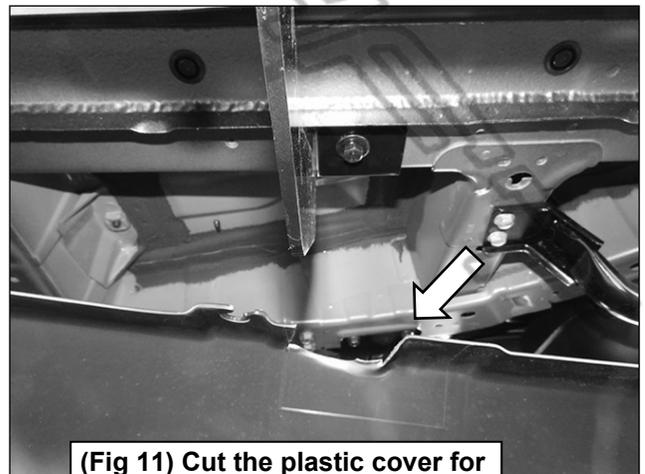
(Fig 11) Cut the plastic cover for the Center Mounting Bracket
