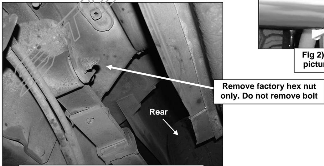
**Fig 3) Driver/left rear leaf spring pivot bolt**
