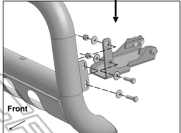
**(Fig 8) Attach Bull Bar to outside of
