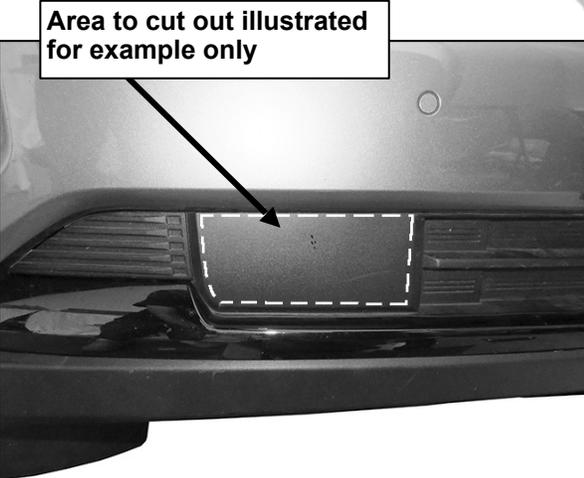
**(Fig 5) Models without tow hooks and without removable covers, (see fig 4), cut openings as required in center plastic panel for Brackets. If necessary, temporarily remove center panel to cut openings. Dashed line represents approximate area to cut. Passenger/right side of center panel pictured**
