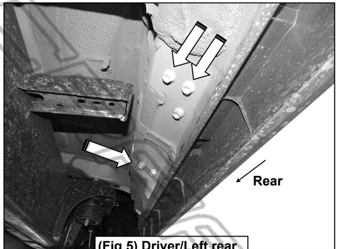
(Fig 5) Driver/Left rear mounting locations
