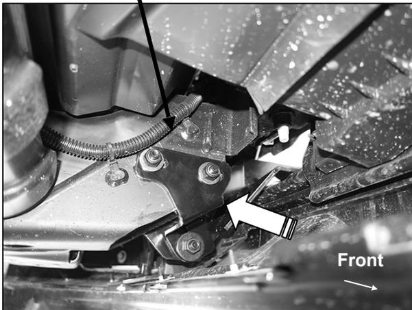
**(Fig 17) Attach driver/left inner Support Bracket to Frame Bracket and Double Bolt Plate in frame (arrow). Driver/left side pictured from below/behind bumper**
