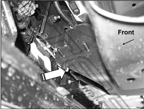
**(Fig 15) Insert Double Bolt Plate through holes in outer side of frame (arrow)**
