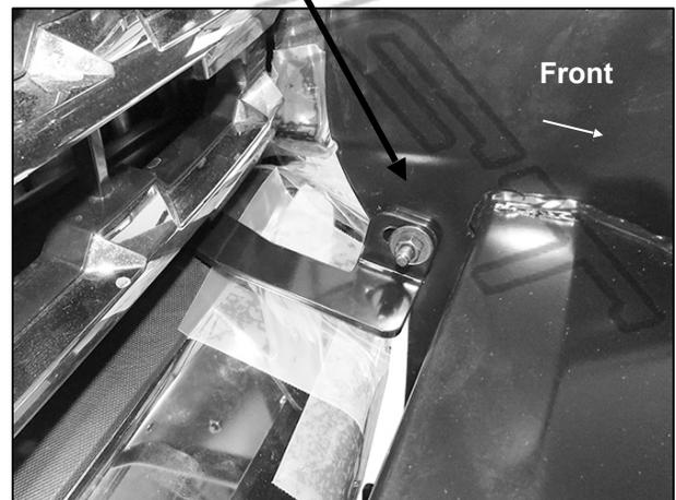
**(Fig 22) Attach Grille Guard to Top Bracket (driver/left side pictured)**
