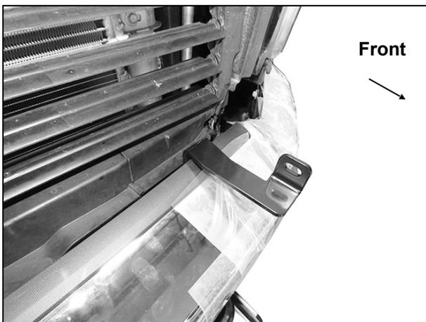
(Fig 10) Reuse top bumper bolt to attach driver/left Top Bracket to top of bumper bracket
