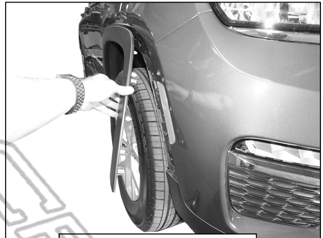
(Fig 4) Gently pry the front of the fender front the bumper
