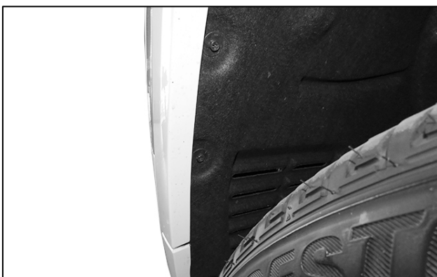
(Fig 1) Remove the hardware connecting the wheel well to the front bumper
