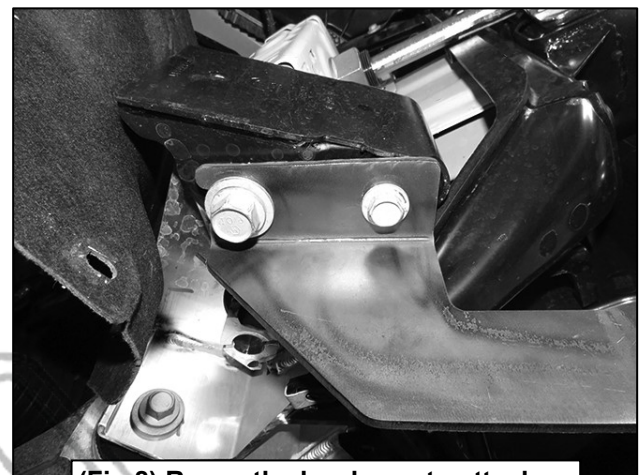
(Fig 8) Reuse the hardware to attach the Passenger/right Mounting Bracket
