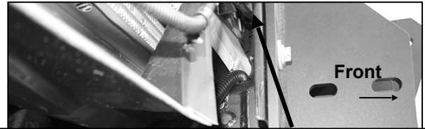
(Fig 19) Right facing Support Bracket installed
