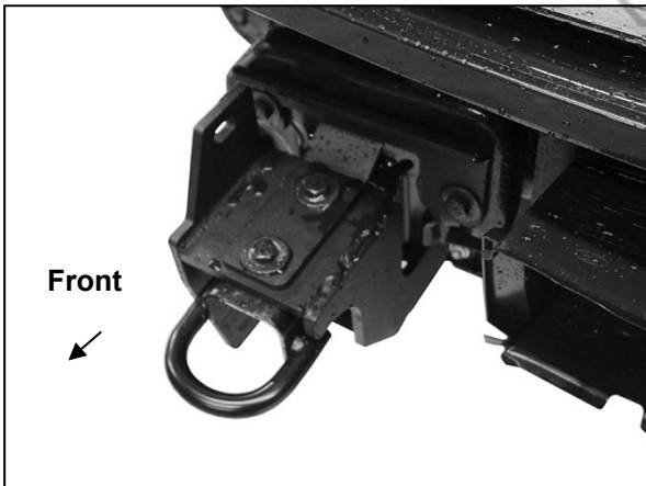
(Fig 12) Passenger/right Frame Bracket and Support Bracket installed with tow hook
