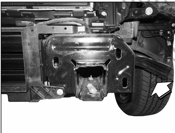
(Fig 6) Remove bumper. Also remove the factory frame extension (arrow-
