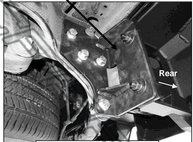
(Fig 19) Bumper installed to Driver/Left Mounting Bracket
