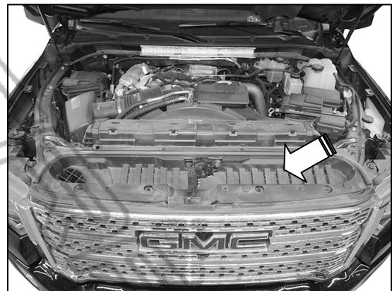
(Fig 2) Remove hood release handle and cover. Reinstall handle. Remove grille. Models equipped with grille camera, pull grille forward and unplug camera
