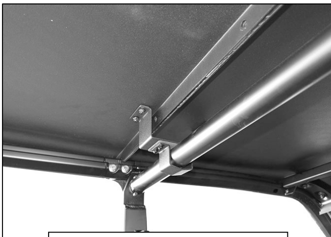
(Fig 18) Center of the Roof Platform attached to the center crossmember
