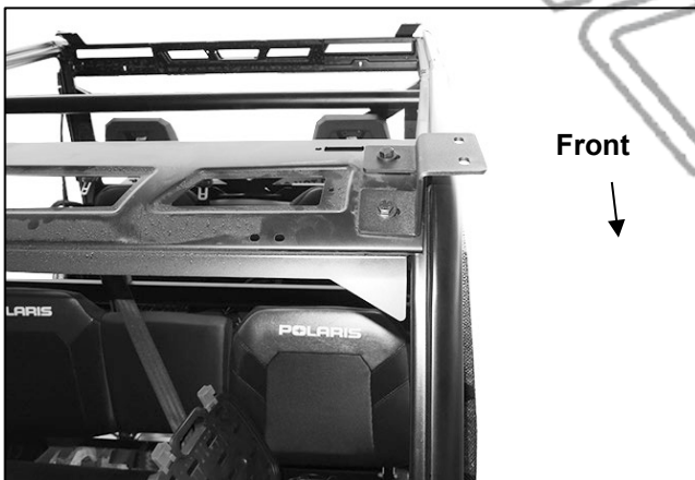
(Fig 5) Driver/Left Front Mounting Bracket attached to the front location
