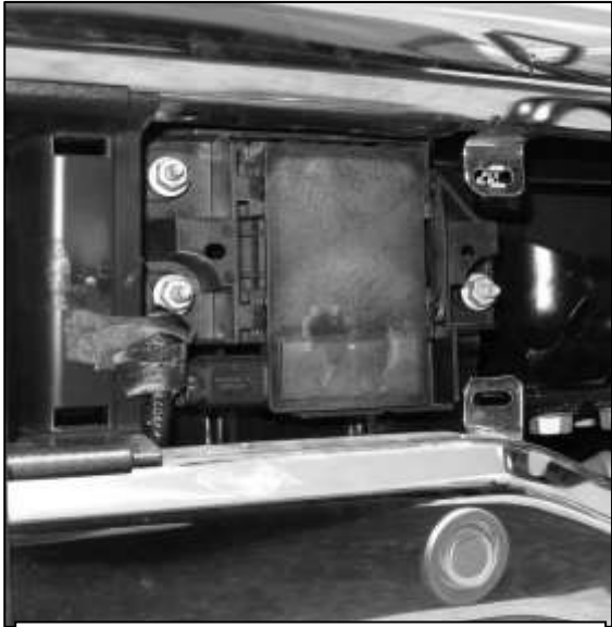
(Fig 17) Remove adaptive cruise control ACC” and parking sensors (if equipped)
