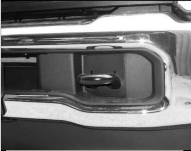
(Fig 3) Remove plastic cover around tow hook
