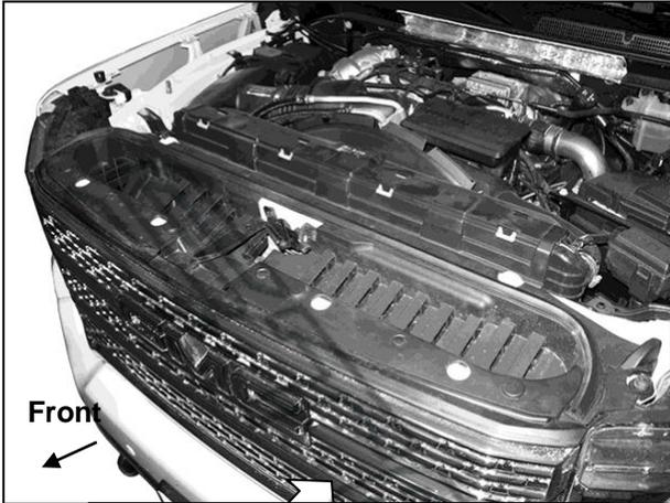
(Fig 1) Open hood and temporarily remove hood release handle
