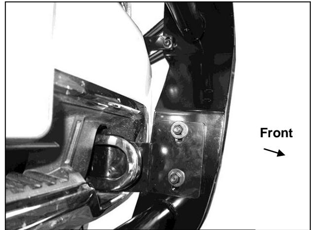
**(Fig 18) Grille Guard installed (driver/left side pictured)**
