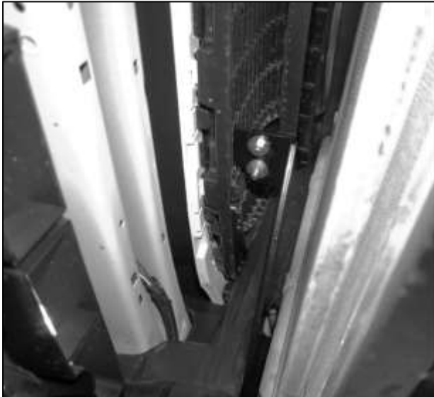
(Fig 9) Outer Support Bracket attached to Lower Support Bracket behind the grille
