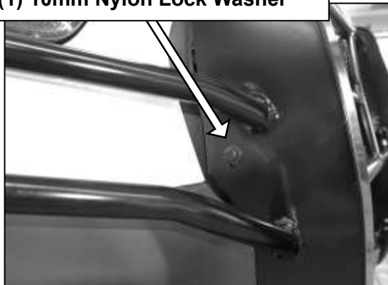
(Fig 15) Attach Grille Guard to Passenger/left Outer Support Bracket
