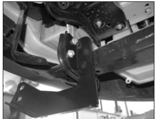
(Fig 12) Passenger/left Frame Bracket Installed
