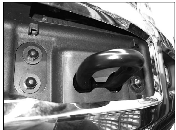
(Fig 4) Remove bumper bolts (driver/left side pictured)
