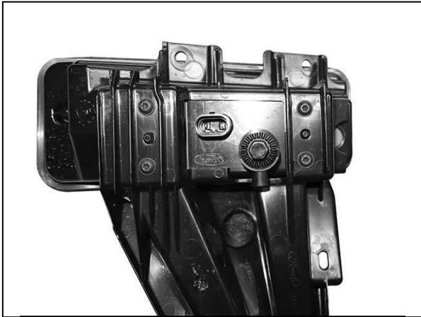
(Fig 14) Remove screws to remove narrow LED fog light from plastic mount
