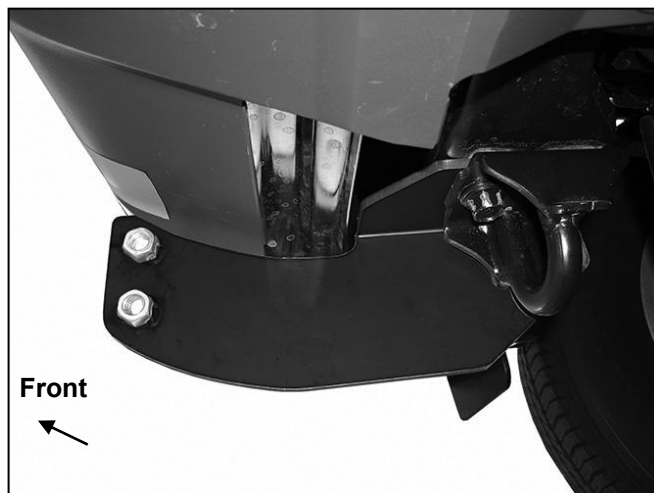
(Fig 11) Reuse factory hex bolts to attach Frame Bracket to bottom of frame (passenger/right side pictured with small tow hook)
