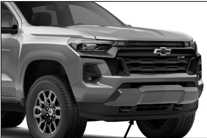
(Fig 1) Vehicles with the plastic air dam can be removed to make install easier
