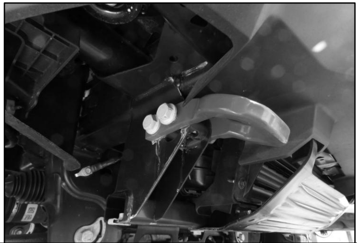
(Fig 4) Tow hooks exposed once air dam/skid plate is removed
