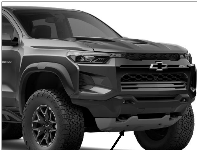
(Fig 2) ZR2 models with skid plates can be removed to make install easier
