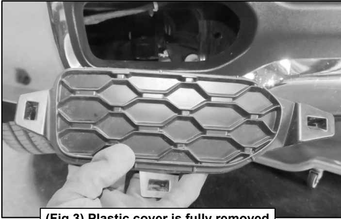
(Fig 3) Plastic cover is fully removed
