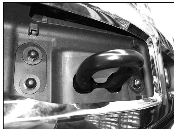
(Fig 4) Remove bumper bolts (driver/left side pictured)
