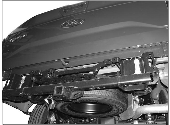
(Fig 14) Reinstall integrated receiver hitch/bracket assembly on models with "HD Towing" package.
