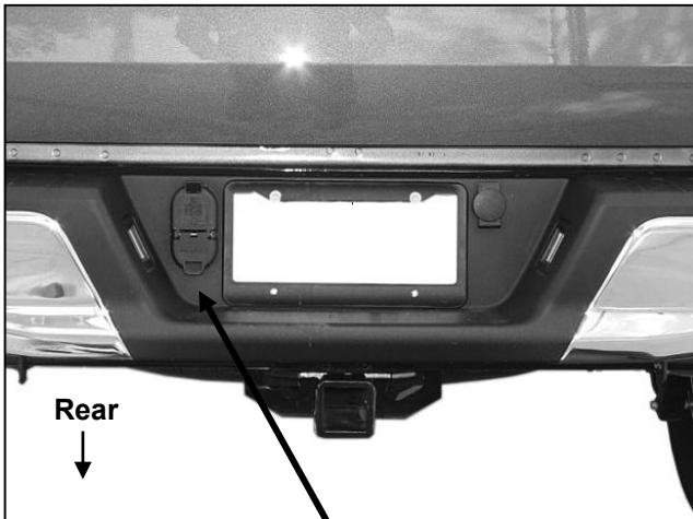
(Fig 1) Unplug and remove 7-wire trailer plug. Remove license plate and spare tire lock.
