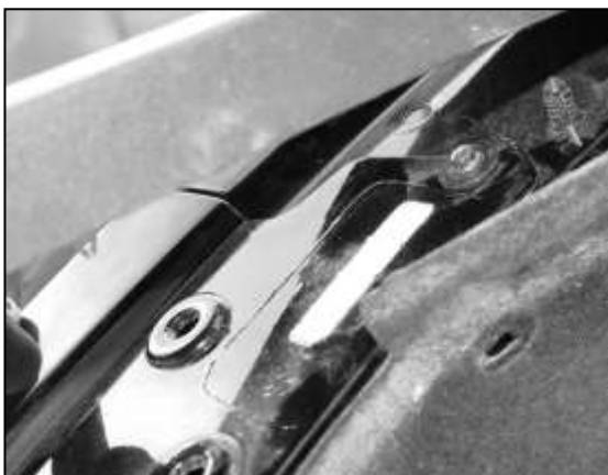
(Fig 3b) 2024-on: Firmly pull flare to expose hex bolt.
