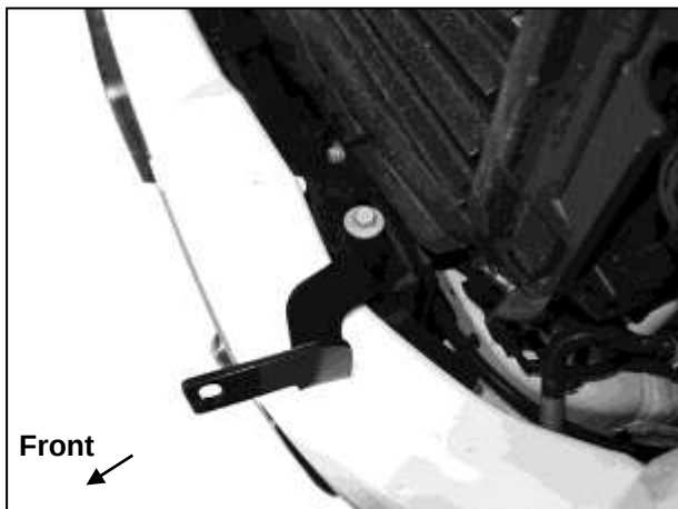
(Fig 7a) 2020-23 models: Reuse bumper bracket bolt to attach Driver/left Top Mounting Bracket to top of frame
