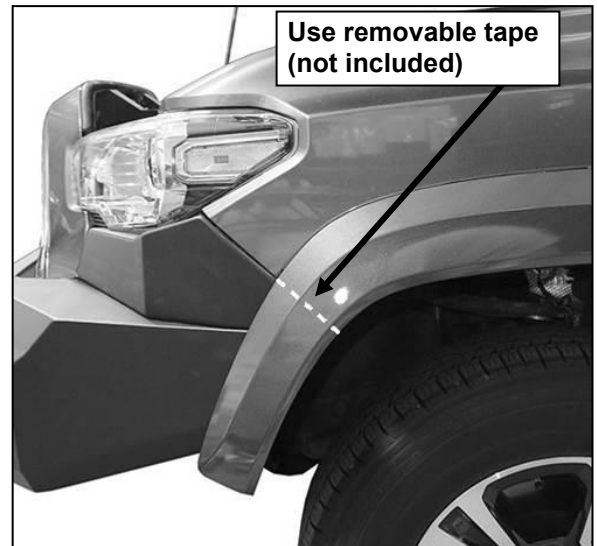
(Fig 23) Cut front end off of the fender flare to match up to Bumper
