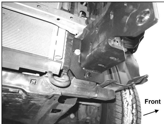
(Fig 11) Attach driver/left Mounting Bracket to end of frame
