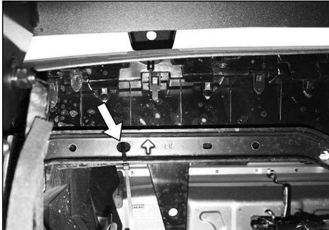
(Fig 9) Use a wire tie (arrow-not included) if needed to attach the bottom of the grille to the inner crossmember
