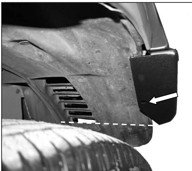
(Fig 24) Secure the fender liner to the bumper using the 6mm button head bolt through the mounting hole shown. Trim liner as necessary.
