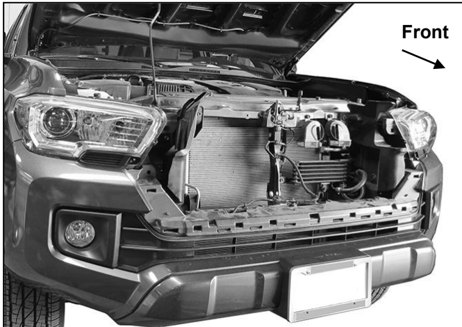
(Fig 3) Remove grille and license plate. Remove plastic bumper cover
