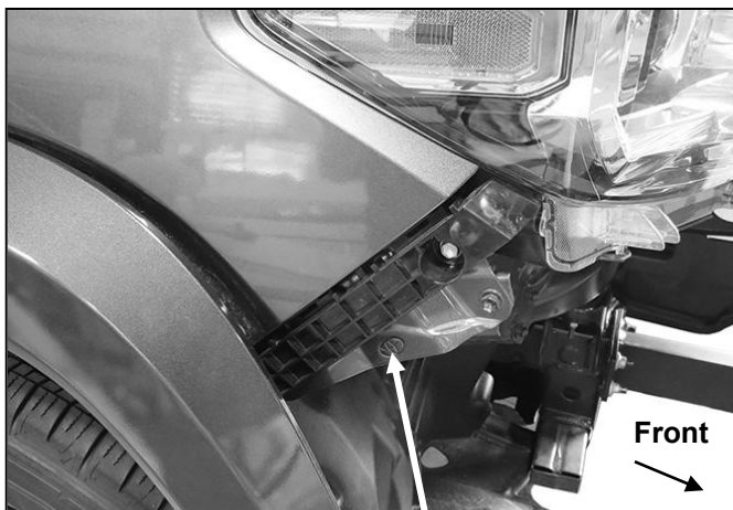
(Fig 5) Remove plastic block (arrow) from front edge of fender. Reinstall hardware to secure headlight
