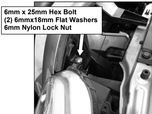
(Fig 8) Replace OE plastic pushpin with supplied hardware
