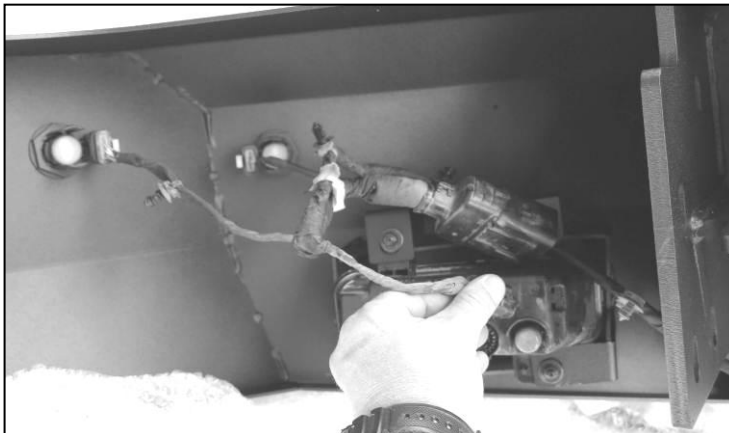
(Fig 18) Use the included Wire Harness Extensions as necessary to reach the parking sensors
