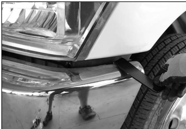
(Fig 13) Starting at the wheel well, slide Top Support bracket between bumper and fascia.
