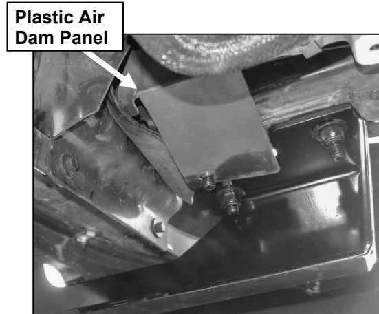
(Fig 16) OPTIONAL: Re-attach plastic air dam to Bolt by sliding over stud
