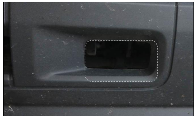
(Fig 8) Hold Frame Bracket up to opening and trim to clear as necessary
