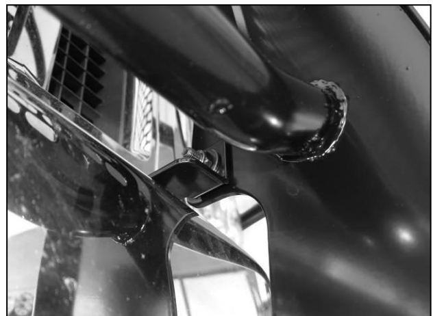
(Fig 20) Driver/Left Top Support Bracket installed
