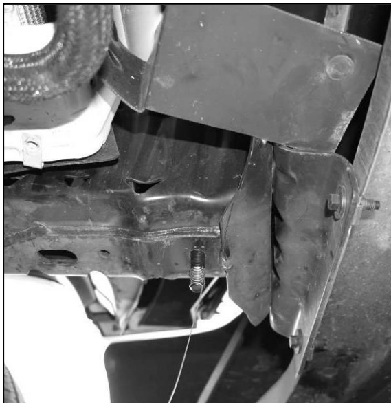
(Fig 5) Pull Bolt Plate fully through frame
