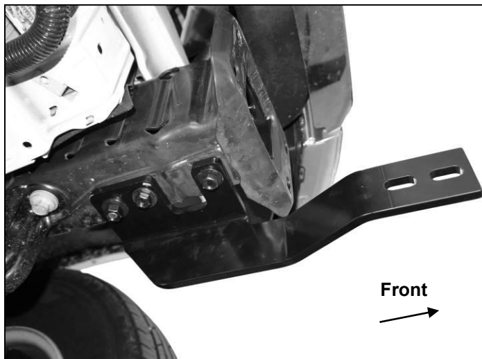
(Fig 6) Support Bracket secured to frame rail
