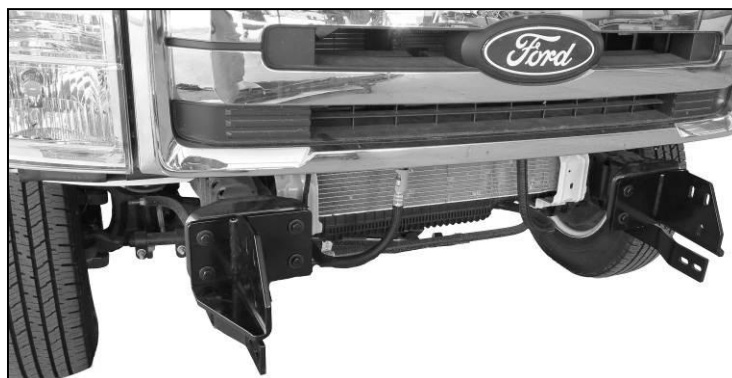
(Fig 8) Frame Bracket and Support Bracket secured to frame rail
