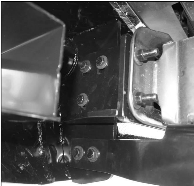
(Fig 15) Bumper Secured to Frame Bracket and Support Bracket
