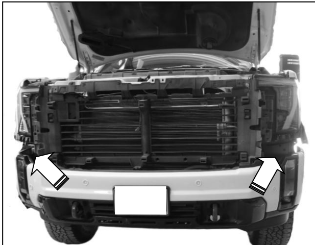
(Fig 5) Once both fascia body panels (arrows) have been loosened, remove grille
