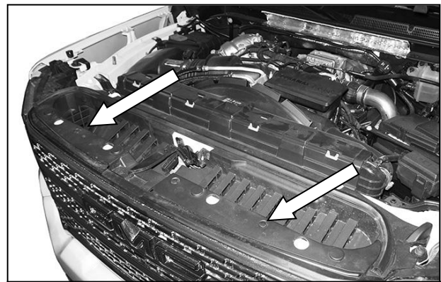
(Fig 2) Remove the plastic pins and cover from the top of the grille and radiator, then temporarily reinstall the hood release
