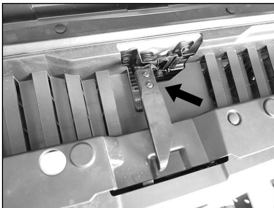
(Fig 1) Remove hood release lever (arrow).
