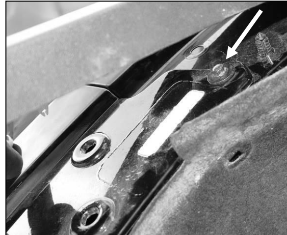
(Fig 4) Firmly pull flare to expose hex bolt.
