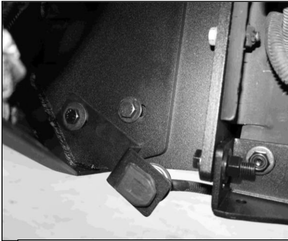
(Fig 26) Driver/left side of Bumper installed (Optional Block Heater installed)
