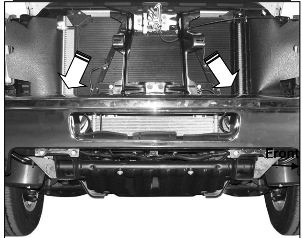
(Fig 2) Remove grille to access bumper bolts. Bumper pictured without lower air dam for instruction purposes-do not remove lower air dam for installation.
